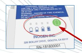
Model # BA-516 16 Cell Battery ~ 13 Hours Run Time
